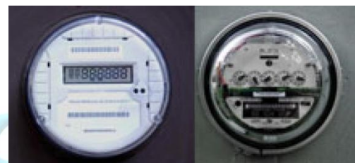
Figure 1: Electromechanical v/s smart meter
