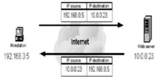
Figure 1: Valid source IP address, illustrates a typical interaction between a workstation with a valid source IP address requesting web pages and the web server executing the requests.
