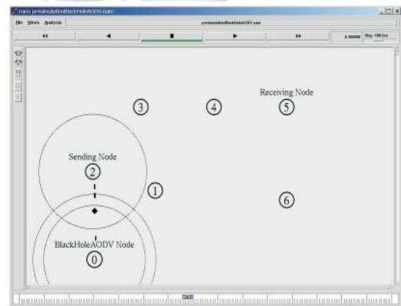
Fig.6. Node 0 (Black Hole Node) absorbs the connection Node 2 to Node 5.
